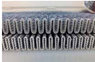
The Filter Media has absorbed water
